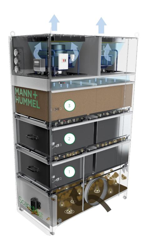
Stages one and two remove 95% of emulsion and 98.5% of neat oil @ 0.4 µm.
