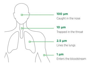
The size of particulate generated by different processes and coolants may vary, but PM1 is by far the most common contaminant.
