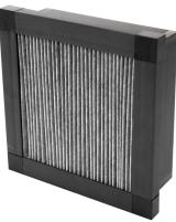
The panel filter itself is environmental firendly, as a result of the easily disposable plastic frame and the syntethic carbon filter media. The frame is rigid, and the media is highly moisture resistant, which makes the whole filter very durable and suitable for demanding environments. The filters large media area assures a very high dust holding capacity, an absorbs gas and odors effectively.
